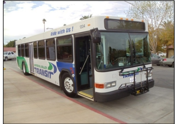
Typical 40-foot city transit bus with wheelchair ramp retracted and bike rack in folded position
